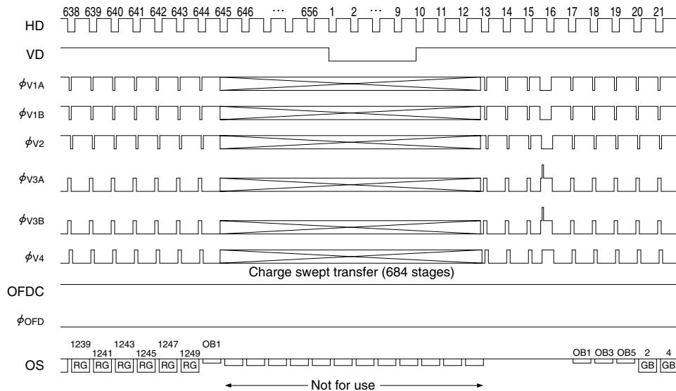
**⑤ VERTICAL TRANSFER TIMING [AT FIRST FIELD ACCUMULATION MODE]**
