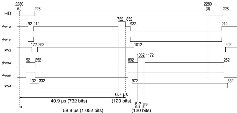
\* Keep over 2.2 μs when vertical transfer clock pulse is overlapping.
