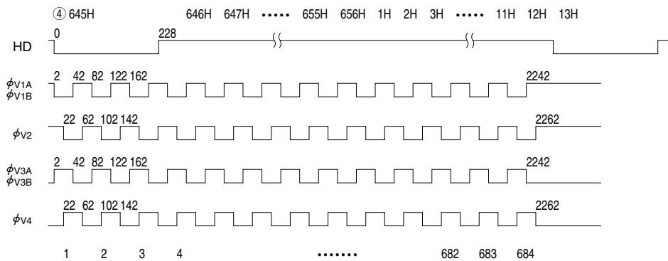
\* Keep over 1.1 μs when vertical transfer clock pulse of charge swept transfer is overlapping.
