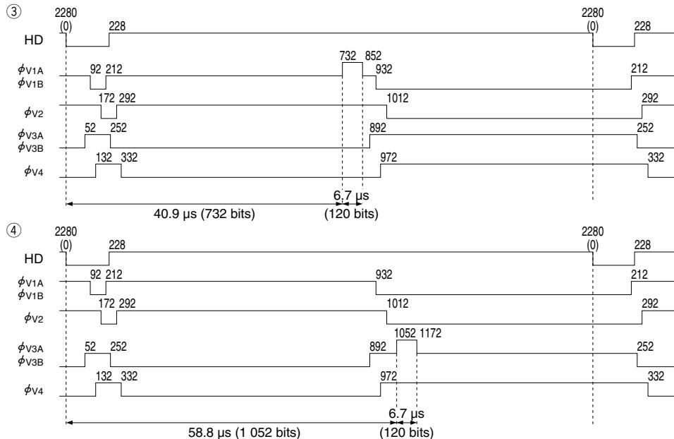
\* Keep over 2.2 μs when vertical transfer clock pulse is overlapping.
