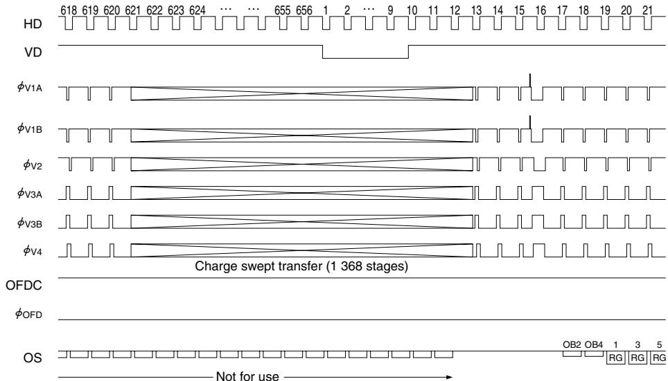
**④ VERTICAL TRANSFER TIMING [FRAME ACCUMULATION MODE]**
